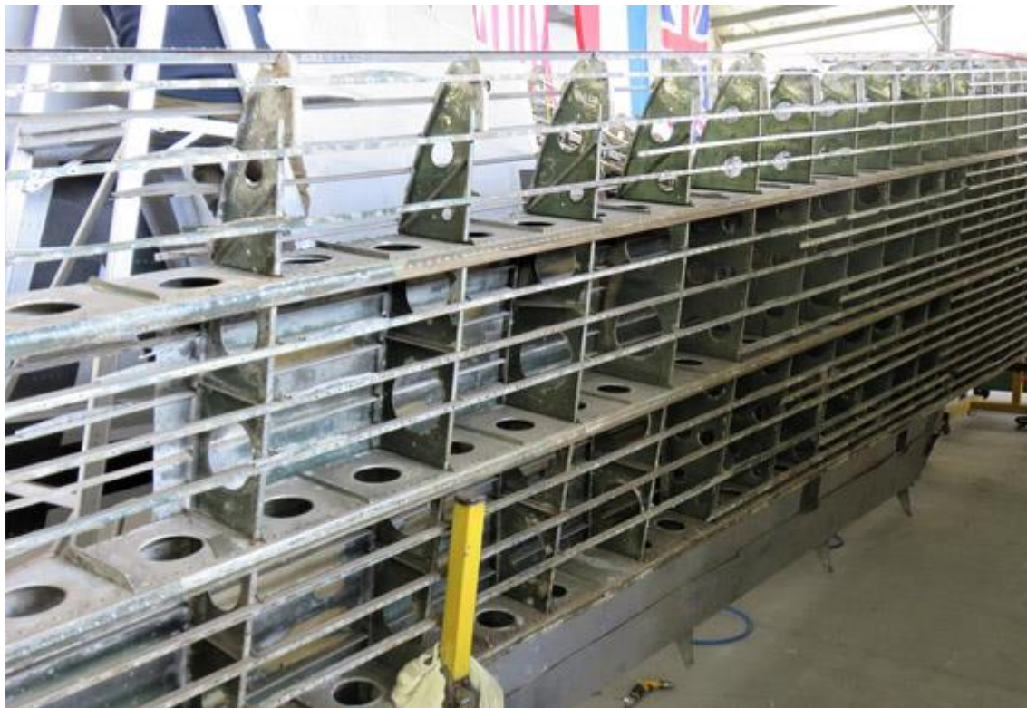
A wing laid bare showing the stringers, most of which will be replaced.
