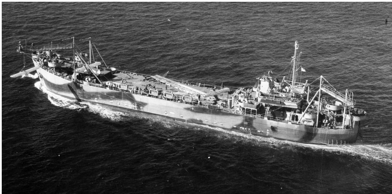
LST-776 during trials off San Diego when fitted with a light catapult amidships (which was removed before the ship entered combat) and the Brodie system.
